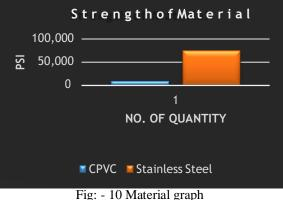
The above graph shows the data between the CPVC and the stainless steel, as it clearly shows that the strength of the stainless steel is quite high, the PSI of the stainless steel is around 75,000
